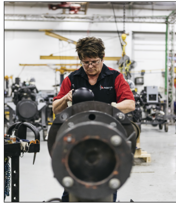
An assembly associate at the AGCO Jackson, MN facility begins building a hydraulic pump that will allow the machinery’s operator to control its movement.
